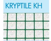
Kryptile KH is our ceramic cube liner. Kryptile KH is available in liners at least 2" (51 mm) thick. Kryptile KH is generally recommended for applications with 15" (381mm) minus rock dropping from a maximum of 8-10+ feet (2.44 - 3.05+ meters).
