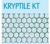
Kryptile KT is the original ceramic hextile liner. The hextile formation is closely gapped to provide superior sliding abrasion resistance in high fines applications, wet or dry. Kryptile KT is generally not recommended for applications where there is impact; it is for slide abrasion only.
