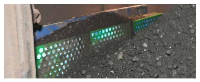
CREATE THE LINER YOU NEED, WHERE YOU NEED IT! Redi-Liner bolt-in 12"x12" panels can be arranged into any wear pattern that is needed. Their unique, simple installation method allows you to replace only what's needed instead of replacing the entire liner.
